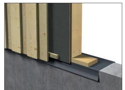
D7. Transition between walls
